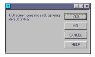
Select **Yes** to generate a default graphical screen. If a default template option has been set in the WorkStation Manager, that template will be applied when the default screen is generated. See WorkStation Manager (Screen Template Options tab). Templates can also be applied from within the Graphic Screen Designer; it is not necessary to set the template option in the WorkStation Manager.
